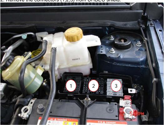
3. Disconnect the connectors(1) from Under Hood Body Electrical Centre shield.
