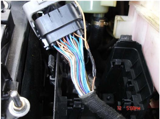
7. Rework all six wires in the same method. And then refit all removed parts.
